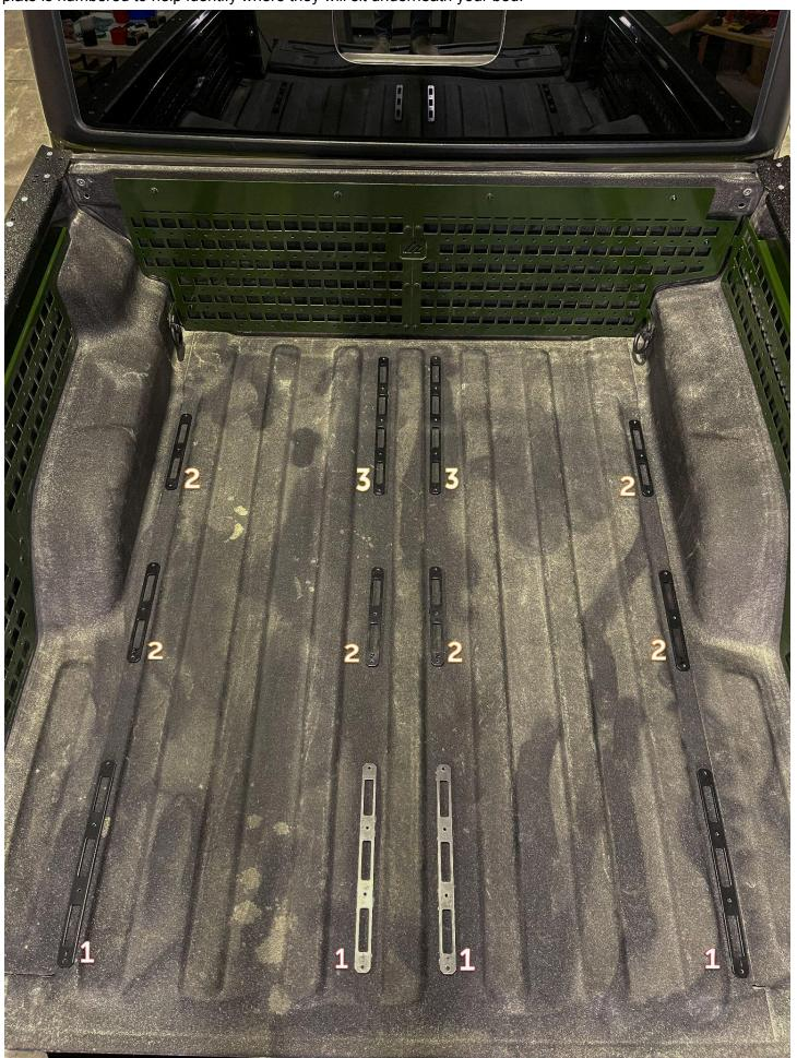
To place the 2 middle #1 nut plates you'll need to remove your spare tire for the install. You can put that spare tire back after the install.
